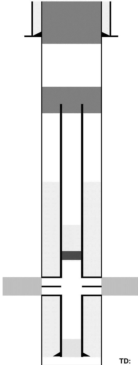
Cut surface casing off 6'-8' below surface.
