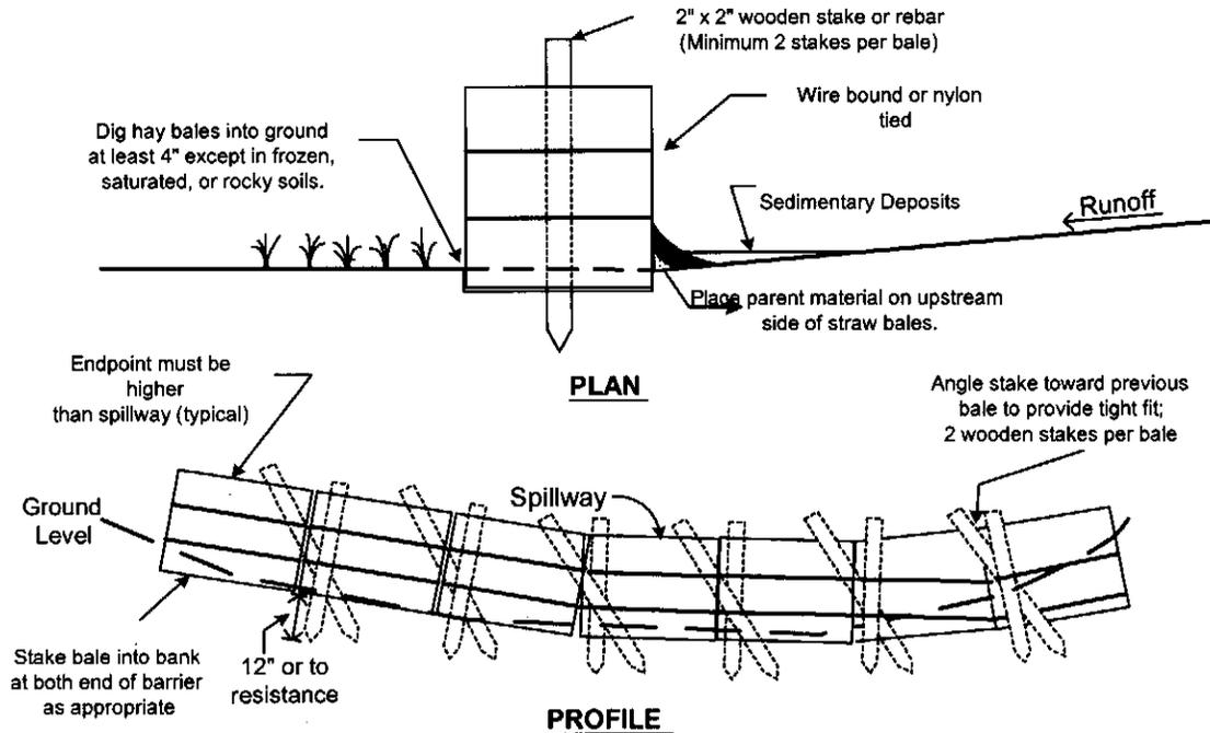
**3.3.1.3 Slope Breaker Construction & Placement**
