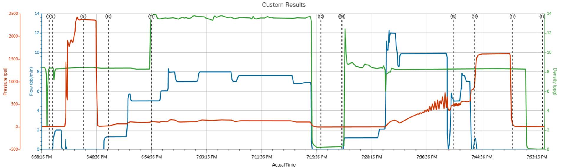
Comb Pump Rate (bbl/min)    DH Density (ppg)    PS Pump Press (psi)
