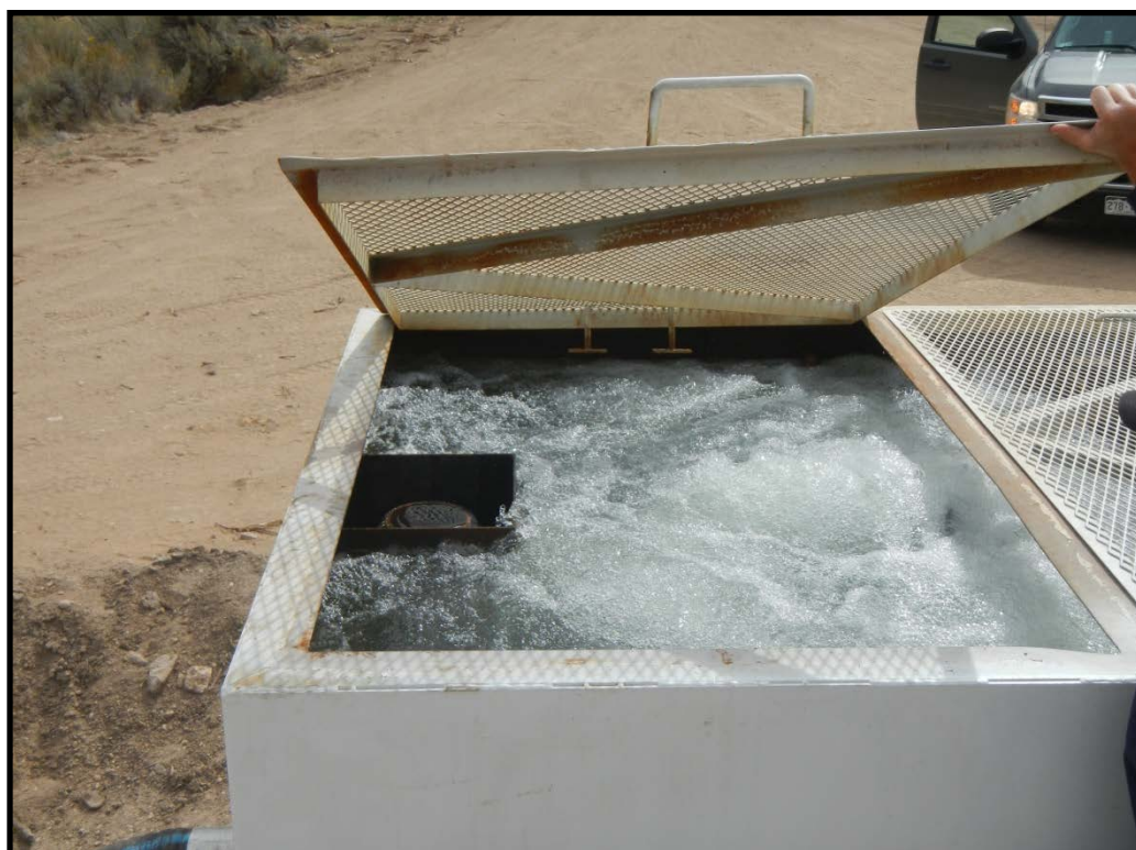
Aerator. Water is discharged back to the creek. Benzene concentration above Table 910-1
