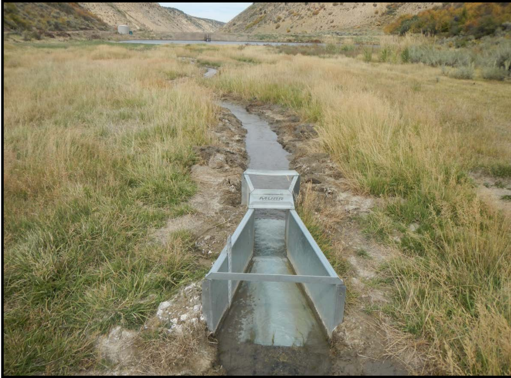
Weir to Measure total discharge to the Stock Pond: Flow from impacted springs plus additional flow from downstream (non-impacted) springs
