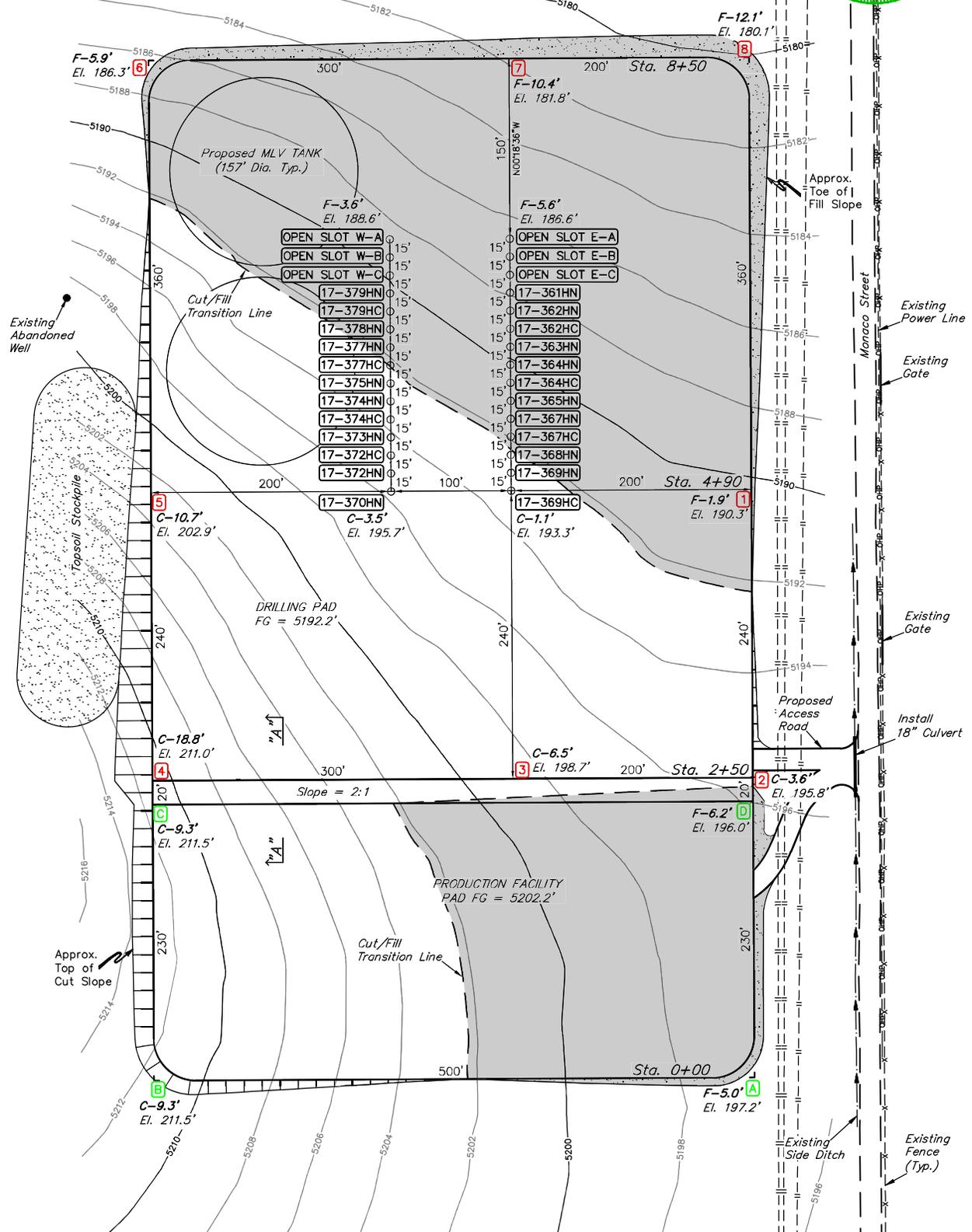
NOTE: Earthwork calculations require a fill @ some of the location stakes for balance. All fill is to be compacted to a minimum of 95% of the maximum dry density obtained by AASHTO method t-99.
