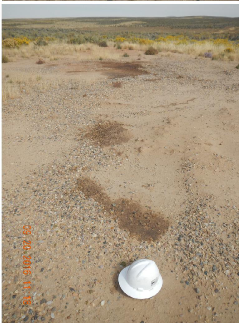
Stained soil in battery area. Hard hat for scale.
