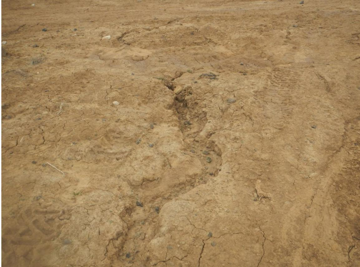
Photo#8: Erosion, channeling, flowing from center of Location to West.
