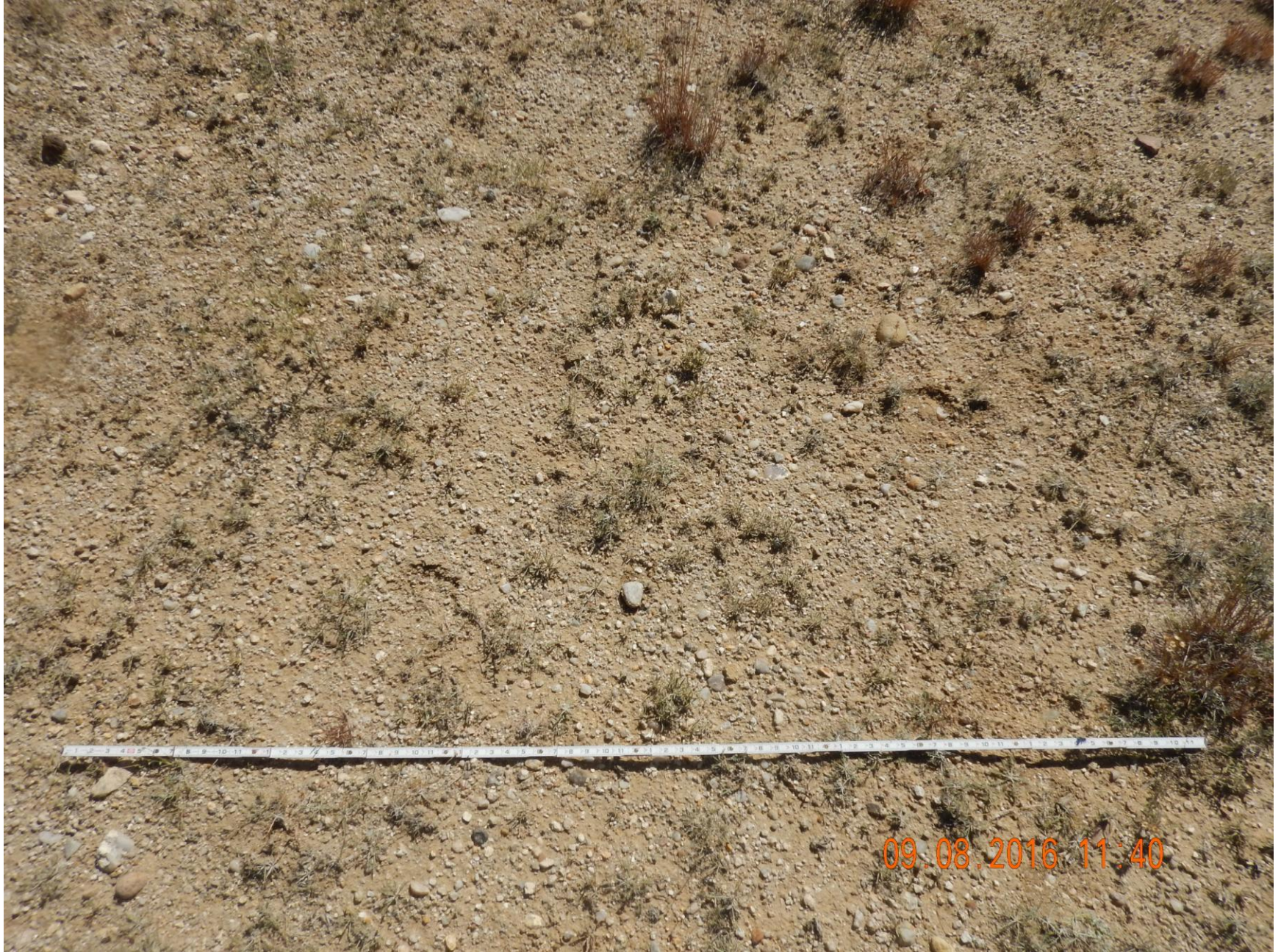
Figure 9: Photo taken from location. Photo shows location has not achieved uniform vegetative cover. 6' measuring stick for reference.
