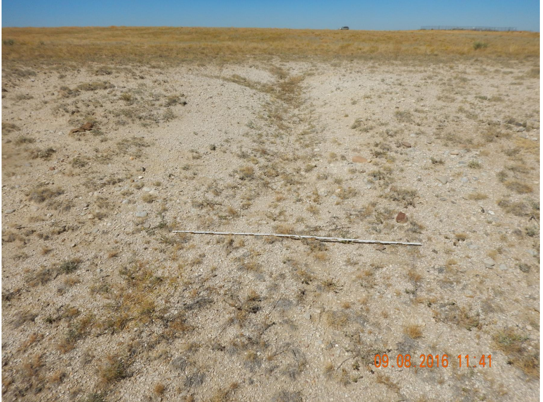
Figure 11: Photo taken from the west end of the location, facing west. Photo shows stormwater erosion occurring on slopes. 6' measuring stick for reference.
