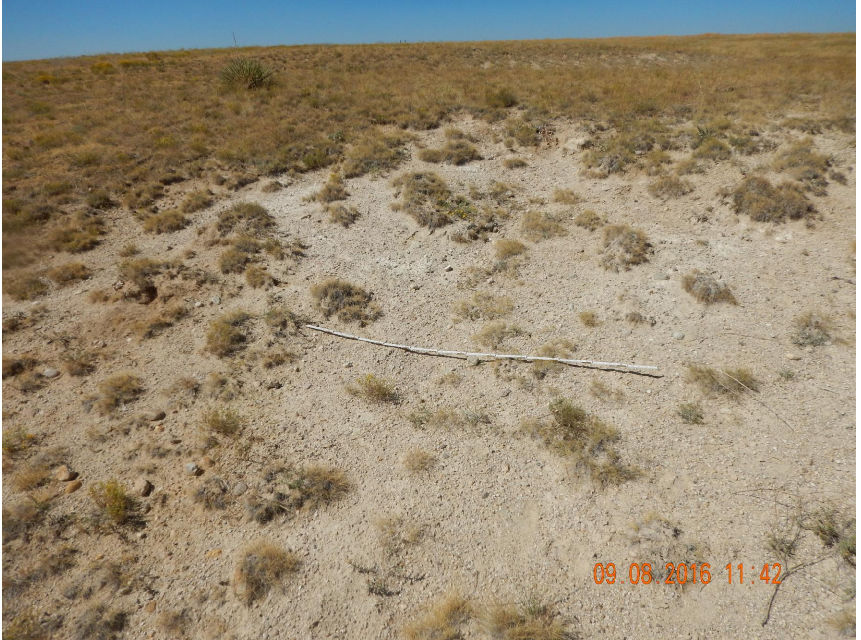
Figure 13: Photo taken from the southwest end of the location, facing southwest. Photo shows stormwater erosion occurring on slopes. 6' measuring stick for reference.
