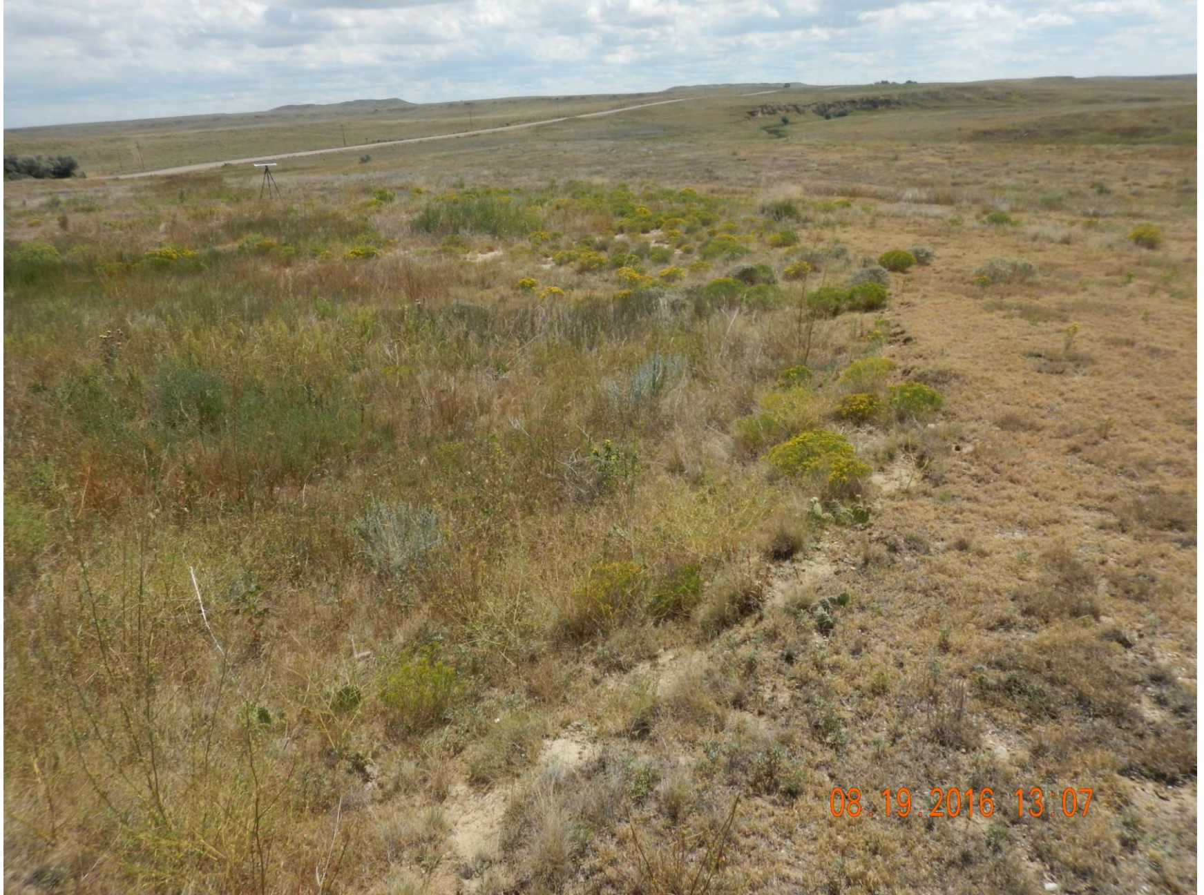
Figure 9: Photo taken from the northwest corner of the location, facing south. Photo shows vegetation over the reclamation area. Note areas of slope seeing erosion. Location has not been re-contoured.
