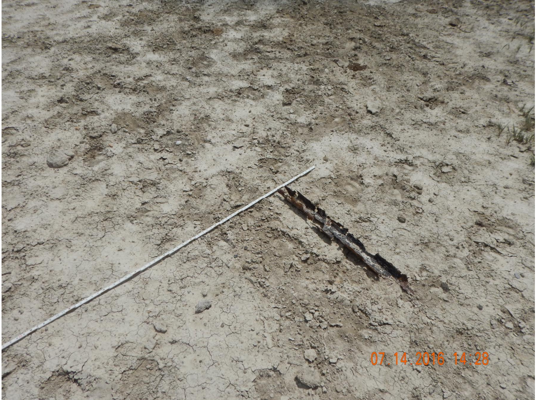
Figure 8: Photo taken from the possible salt kill. Photo shows pipe equipment and debris found in the possible salt kill. 6' measuring stick for reference.
