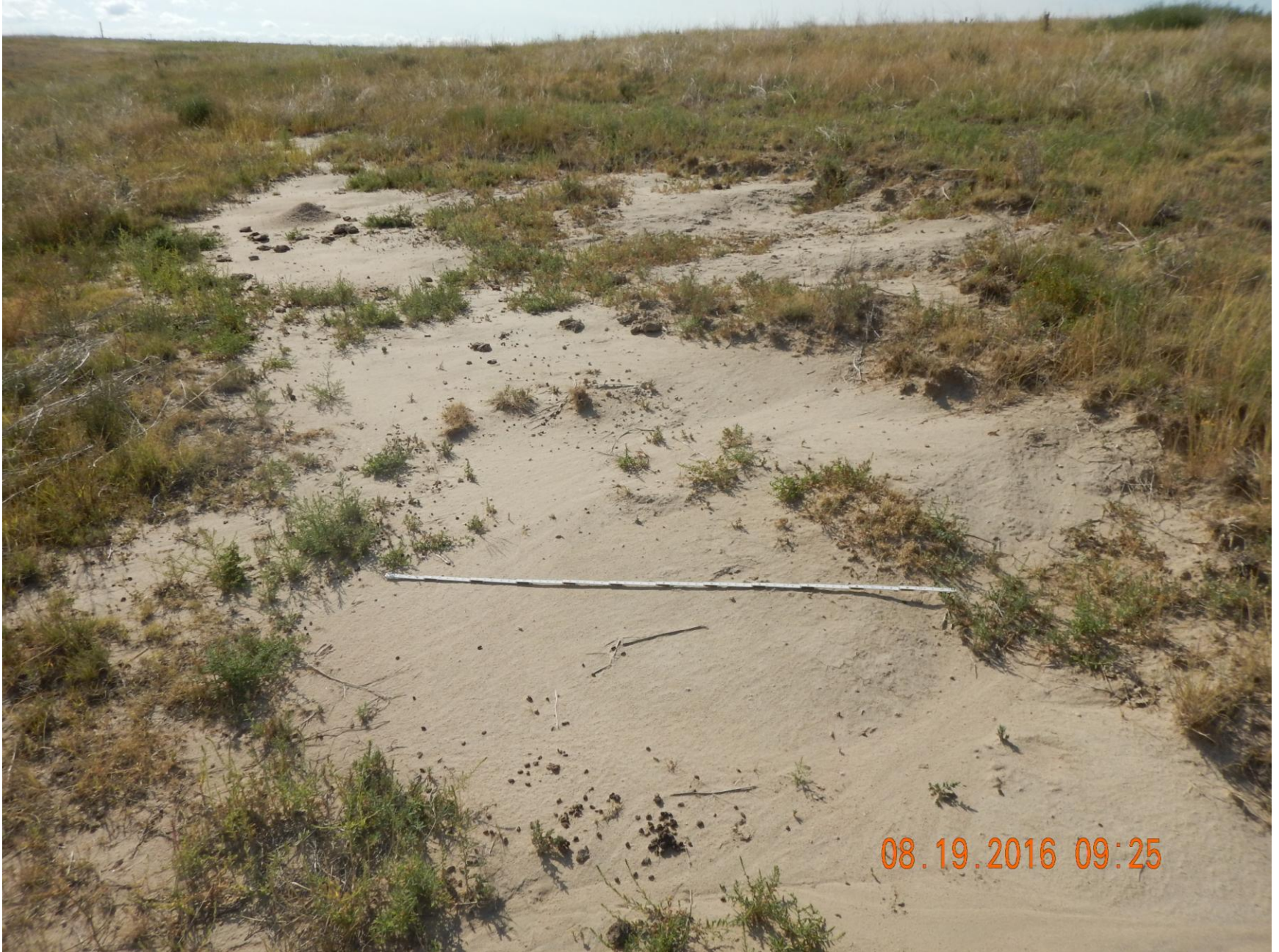
Figure 6: Photo taken from the location. Photo shows large bare areas on location where erosion is occurring. 6' measuring stick for reference.
