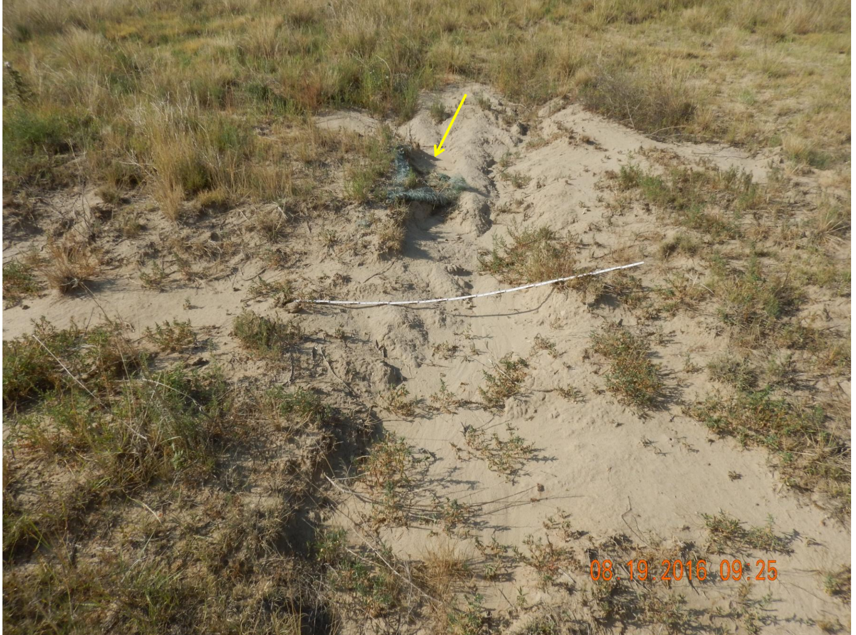
Figure 5: Photo taken from the location. Photo shows large bare areas on location where erosion is occurring. 6' measuring stick for reference. Arrow shows remnants of a sediment control blanket no longer in proper functioning condition, and is now debris.
