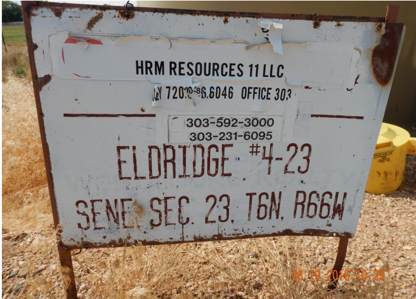
Photo 1. Photo taken of PR well sign for API 123-13177. Emergency contact on sign is not legible and not complete.
