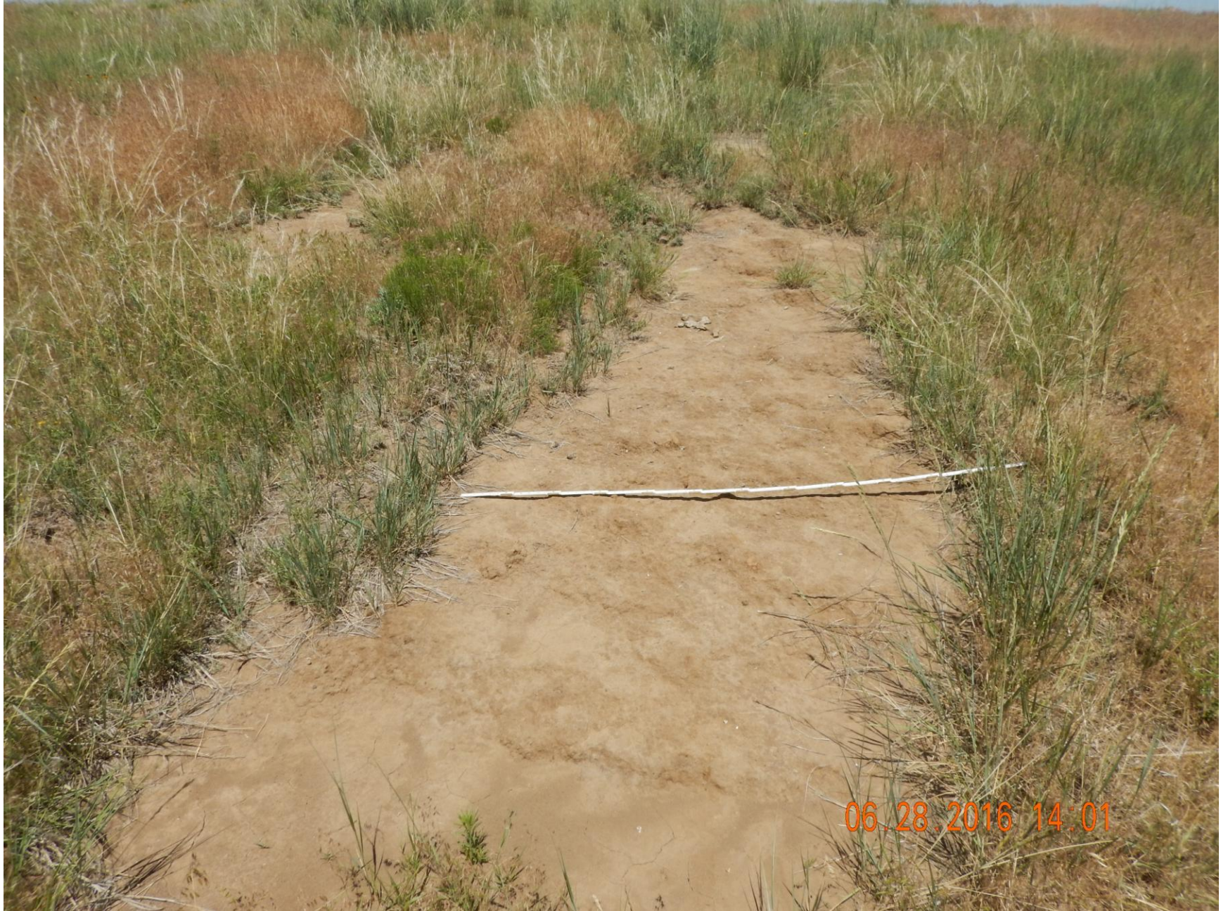
Figure 12: Photo taken from within the fenced remediation area. Photo shows remediation has not achieved uniform vegetative cover per reclamation regulations. 6' measuring stick for reference.
