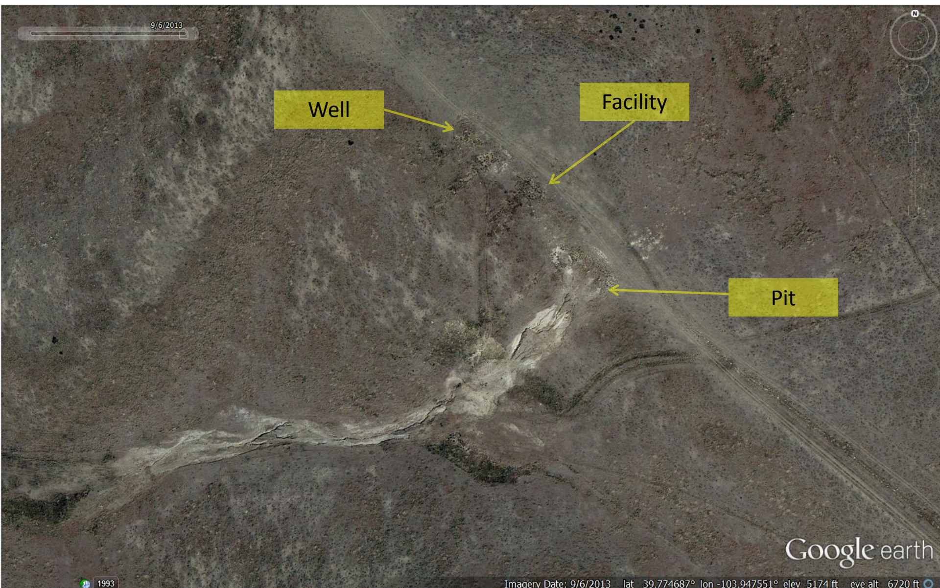
Figure 2: 9/6/2013 aerial imagery of location. Note areas of degradation (southern and northern), and an area that has been fenced off
