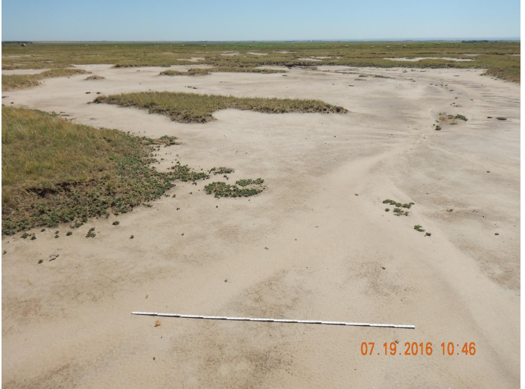
Figure 22: Photo taken from the south central area of the location, facing east. Photo shows areas of degradation due to stormwater erosion and possible salt kill from the location. 6' measuring stick for reference
