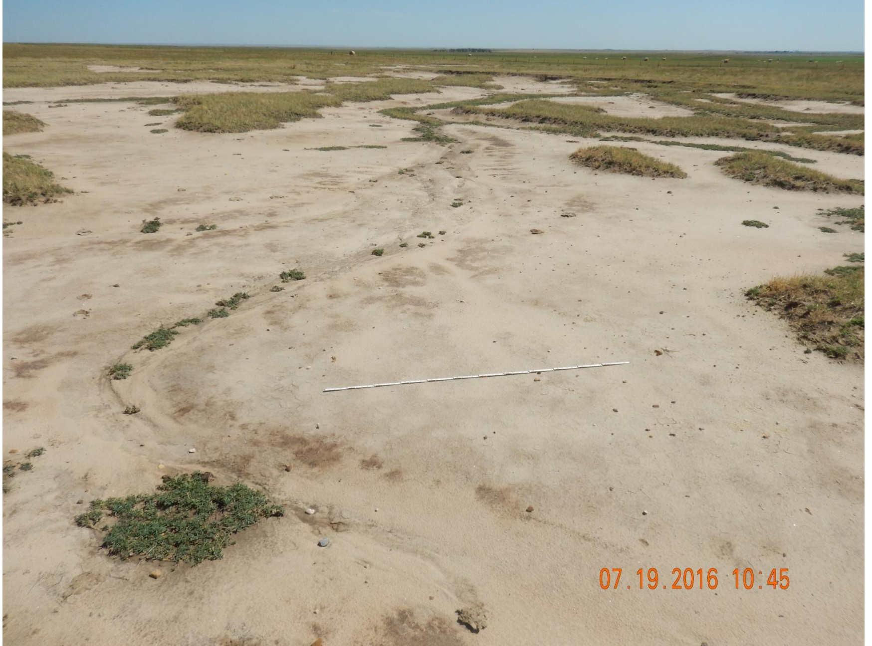
Figure 21: Photo taken from the north central area of the location, facing east. Photo shows areas of degradation due to stormwater erosion and possible salt kill from the location. 6' measuring stick for reference
