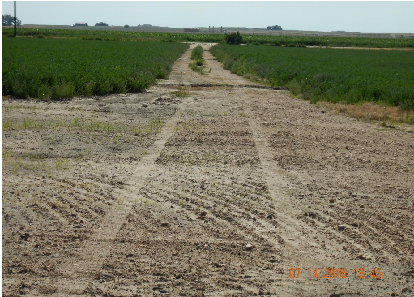
Photo 5. Photo taken from the central tank battery location, facing West. Evidence of seeding is noticeable. However, gravel remains and compaction alleviation was not completed making near impossible for anything to grow.
