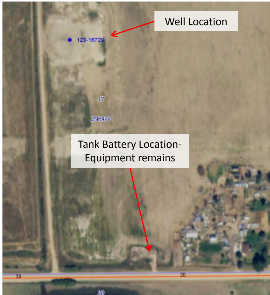
Photo 1. 2015 aerial imagery using COGCC GISOnline database, illustrating the well location and tank battery location where equipment remains.
