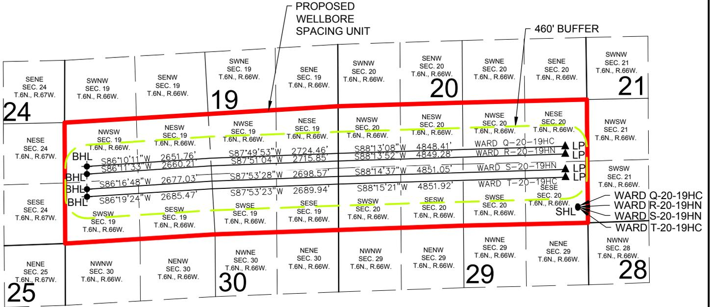
WELL **WARD Q-20-19HC** TO BE LOCATED 364' FSL AND 213' FEL, SEC. 20, T6N, R66W
