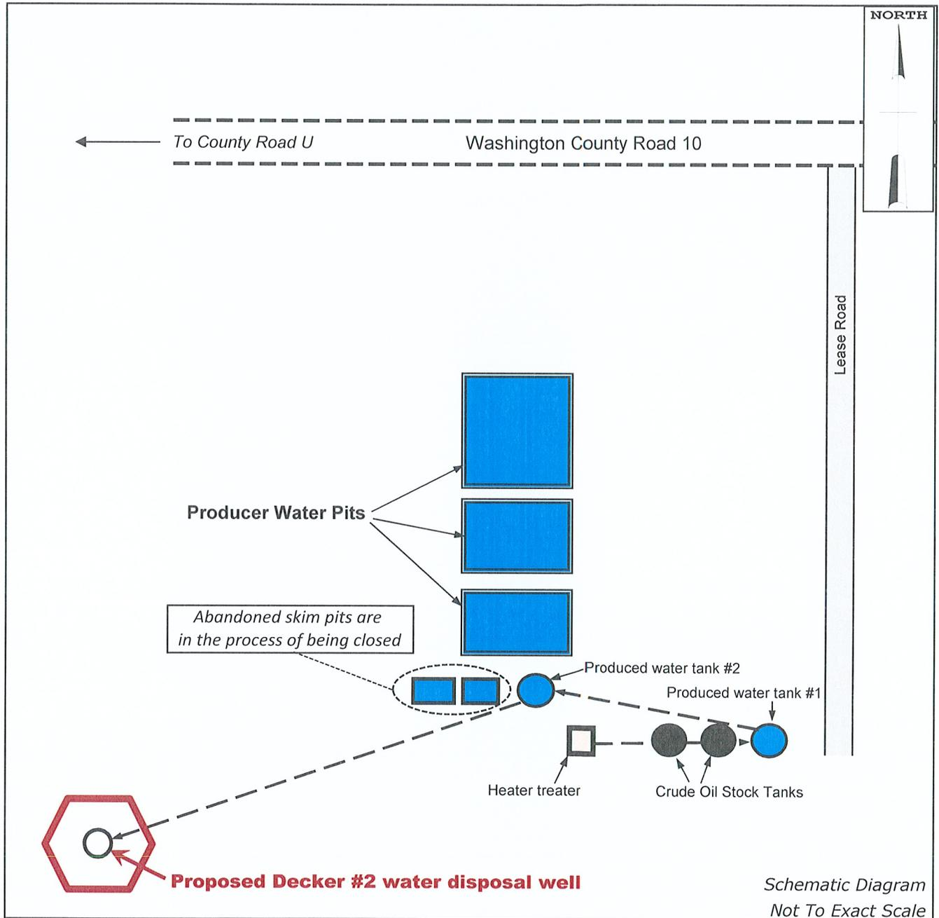
**NOTE:** Produced water will go from Heater Treater to water tank #1, then from water tank #1 to water tank #2, then from water tank #2 to the Decker #2 well.
