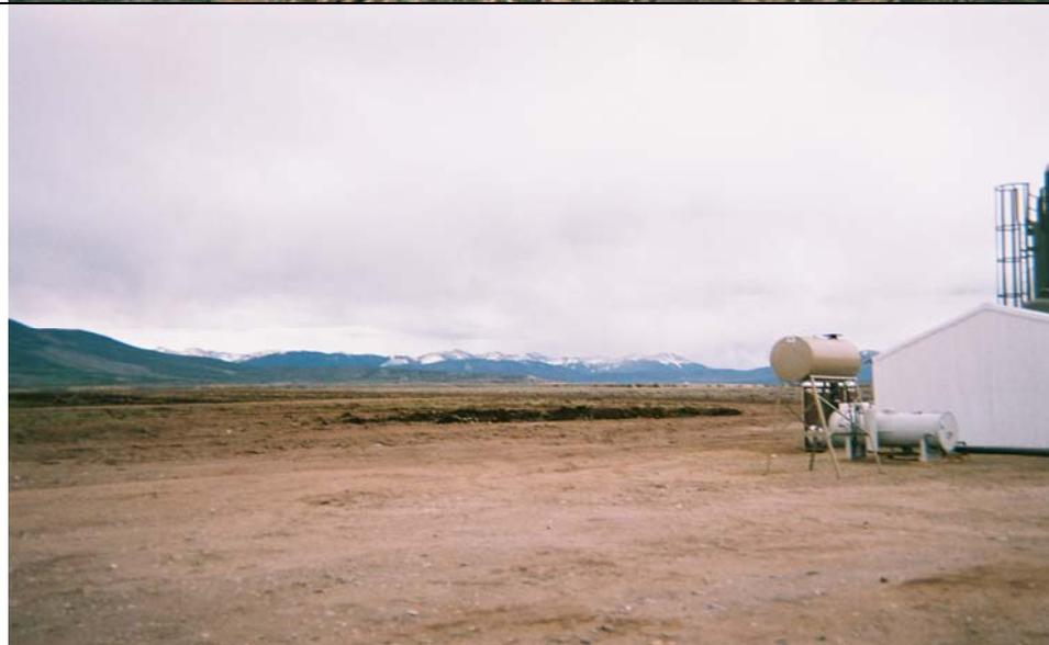
**Subject:** Photograph shows the stockpiled vegetation and stained soils and the vertical separator (right). Soil sample SS10 was collected from the stockpiled vegetation and soils located within an earthen containment berm.
