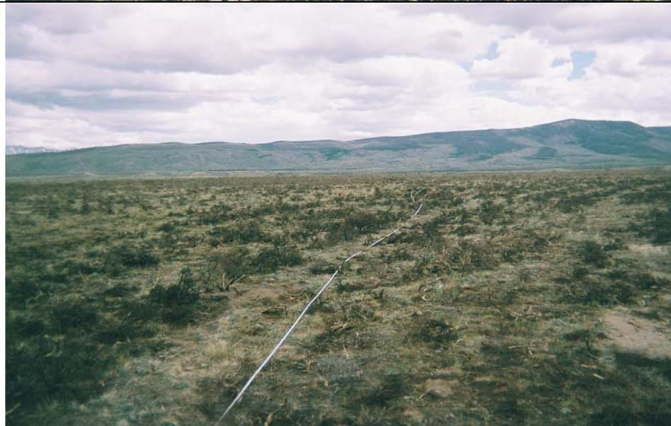
**Subject:** Photograph shows the approximate centerline of the release looking to the east of the Fuqua 18-15 well pad. The extent of primary impact and the soil sample locations were measured using fiberglass tape measures. The photograph was taken near the locations of SS7 (right – south ~25 feet) and SS8 (left – north ~15 feet) from the release centerline.
