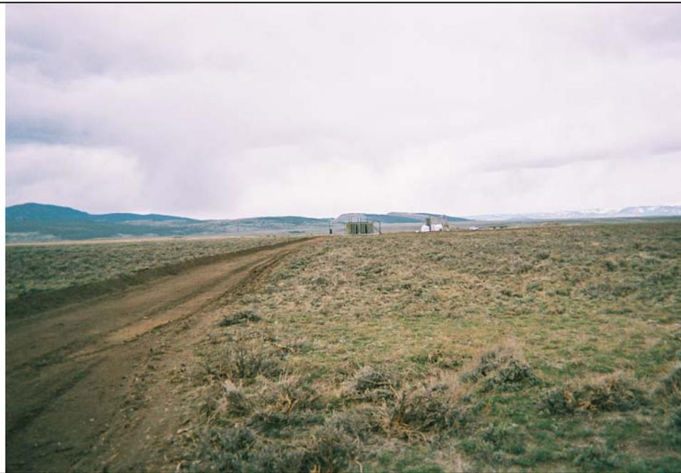
**Subject:** Photograph shows the Fuqua 18-15 well pad from the southeast corner of the fire break. The soils and vegetation were not observed to be impacted out this far; however, there were “fingers” and spots of staining that extended from the primary impact area that are included within the extent of the fire break.
