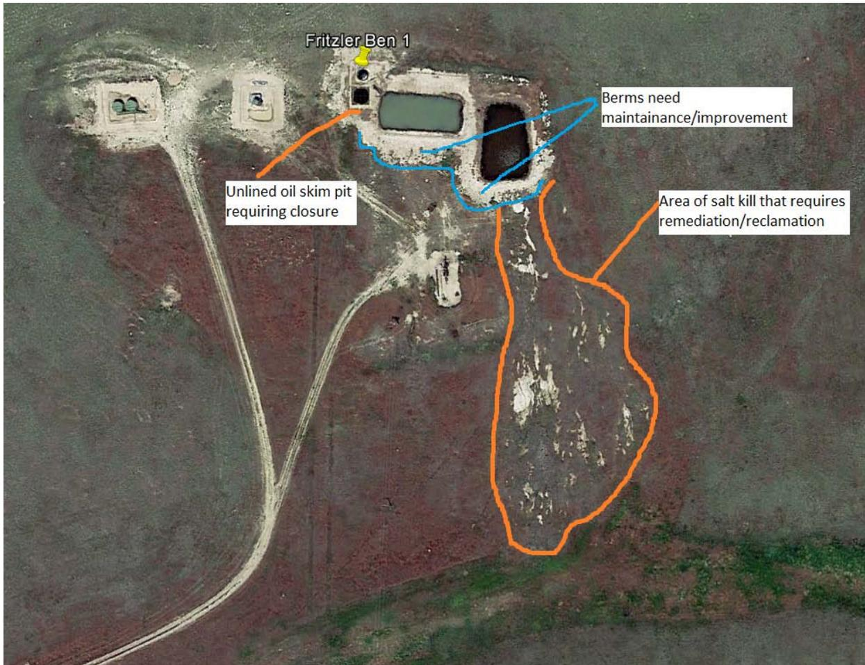
Southern produced water pit berms require maintenance and erosion control.
