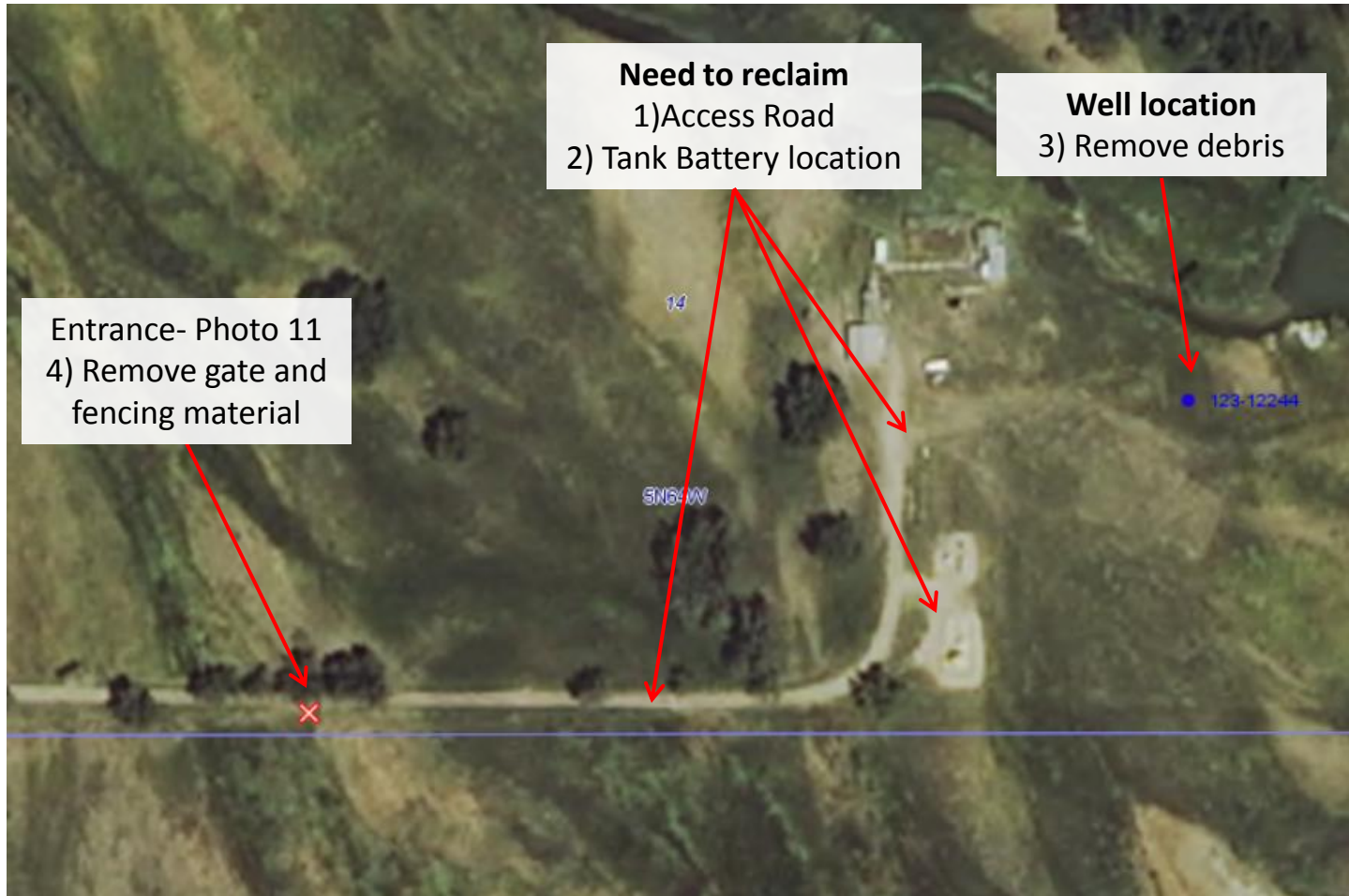
Photo 1. 2013 aerial imagery using COGCC GISOnline, illustrating total areas that have not been reclaimed per Rule 1004 and debris left behind.
