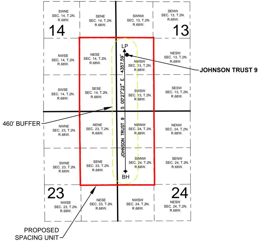
WELL **JOHNSON TRUST 9** TO BE LOCATED 2041' FSL AND 388' FWL, SEC. 13, T2N, R68W
