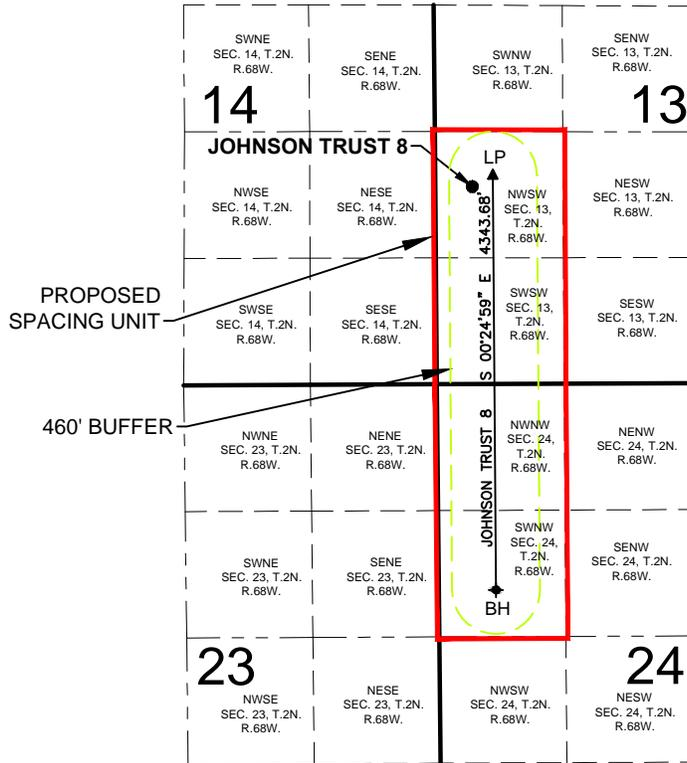
WELL **JOHNSON TRUST 8** TO BE LOCATED 2069' FSL AND 388' FWL, SEC. 13, T2N, R68W
