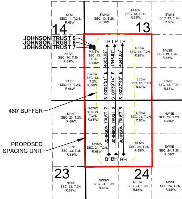
WELL **JOHNSON TRUST 5** TO BE LOCATED 2153' FSL AND 389' FWL, SEC. 13, T2N, R68W
