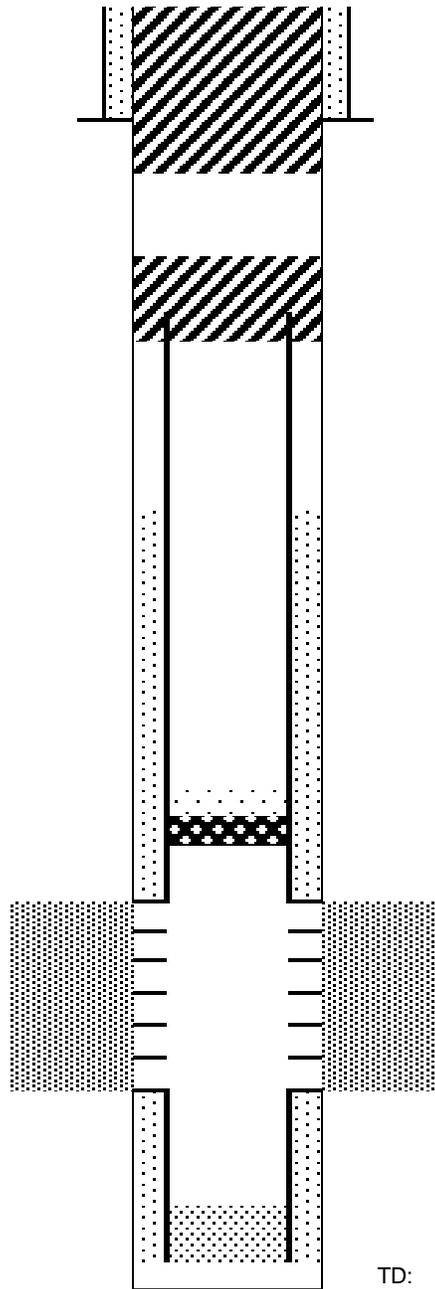
Cut surface casing off 6'-8' below surface.
