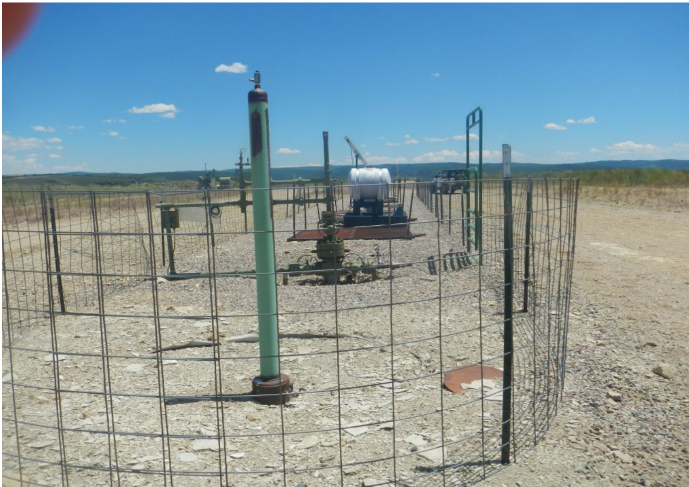
Photo#1: Marker Identifying P&A Well on this Active Location.
