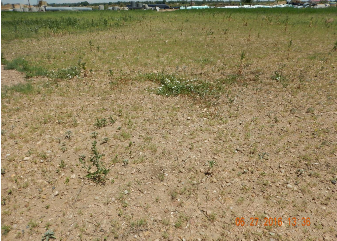
Photo 5. Photo taken from well location, facing East. Need to reclaim location per Rule 1004. A seeding attempt was made but gravel was not removed preventing proper vegetative establishment.
