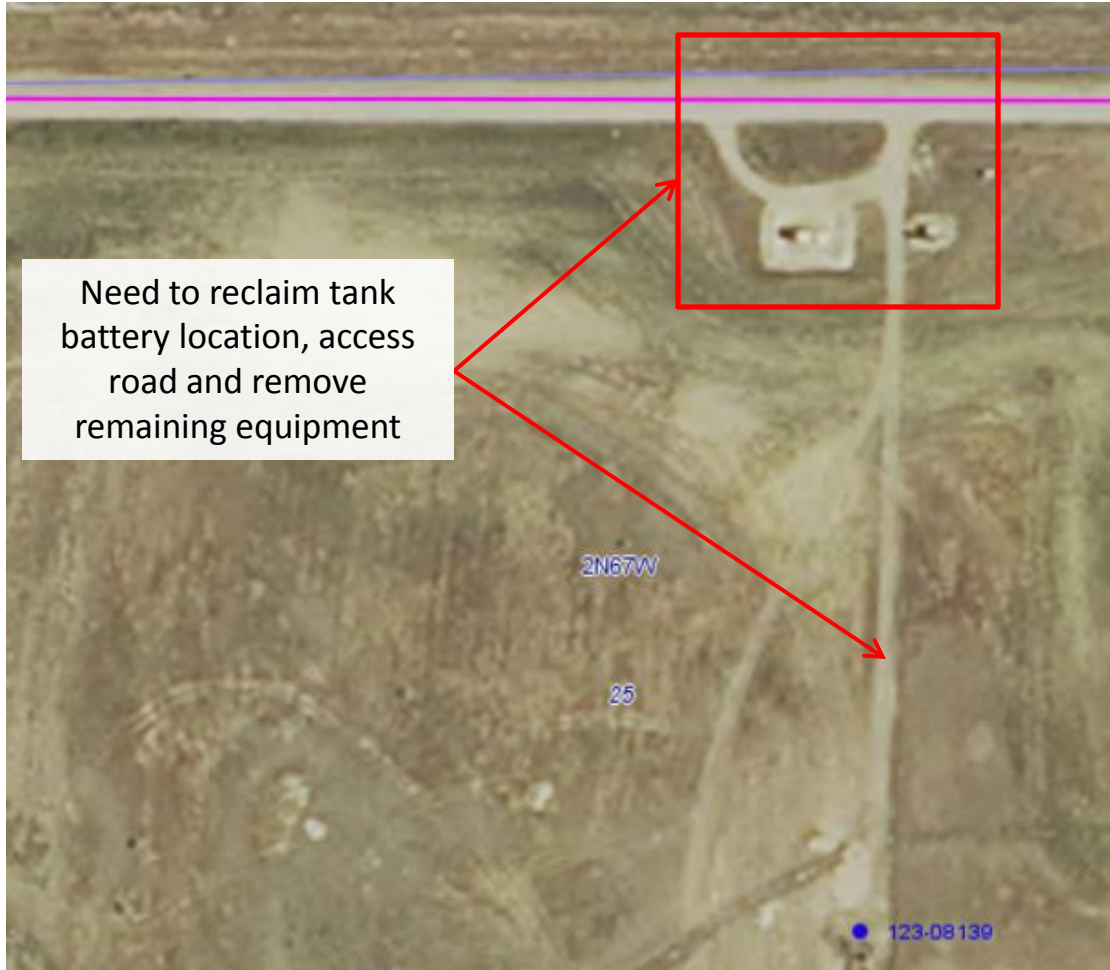
Photo 1. Aerial imagery taken 2013 using COGCC GISOnline, illustrating areas that still have not been reclaimed per Rule 1004.
