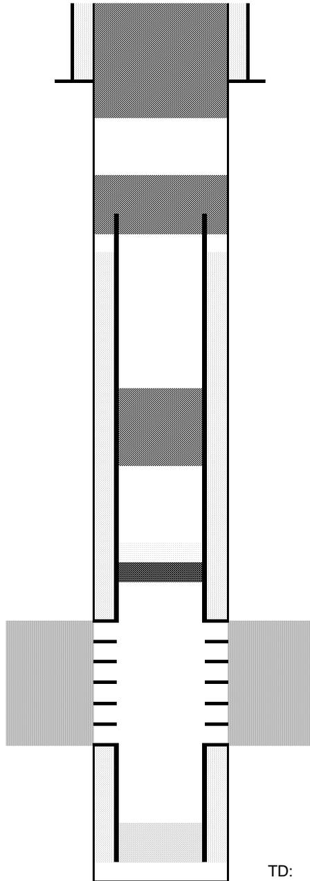
Cut surface casing off 6'-8' below surface.
