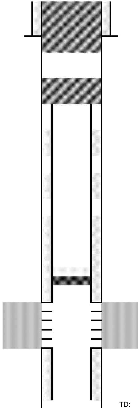
Cut surface casing off 6'-8' below surface.
