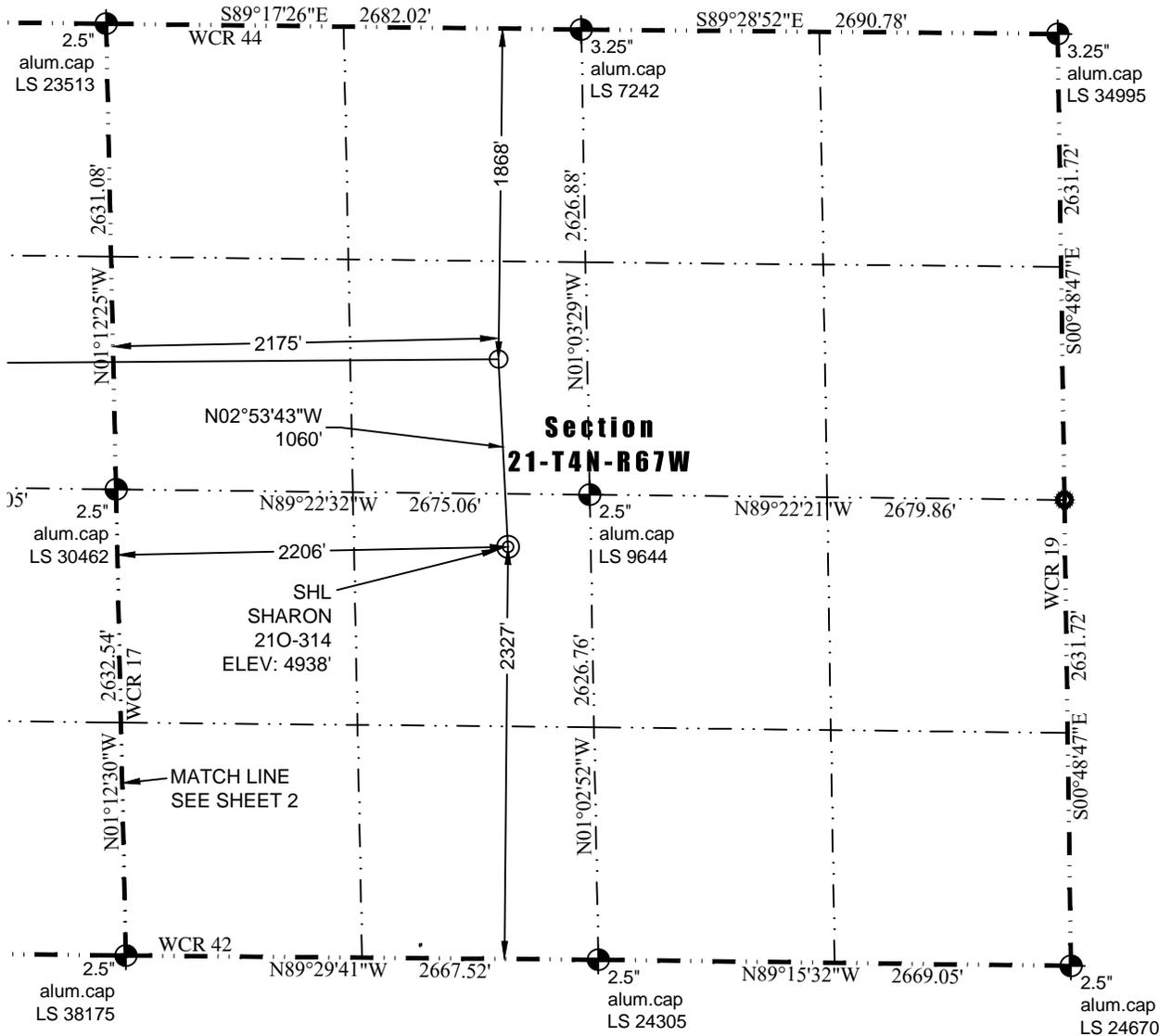
In accordance with a request from Mac Neumann of PDC Energy, Inc., Washburn Land Surveying, LLC has determined the location of the **SHARON 210-314** well site to be SHL: 2327' FSL and 2206' FWL, (BHL: 1990' FNL and 500' FWL), as measured at ninety (90) degrees from the section lines of Sections 21 and 20, Township 4 North, Range 67 West of the 6th Principal Meridian, Weld County Colorado.
