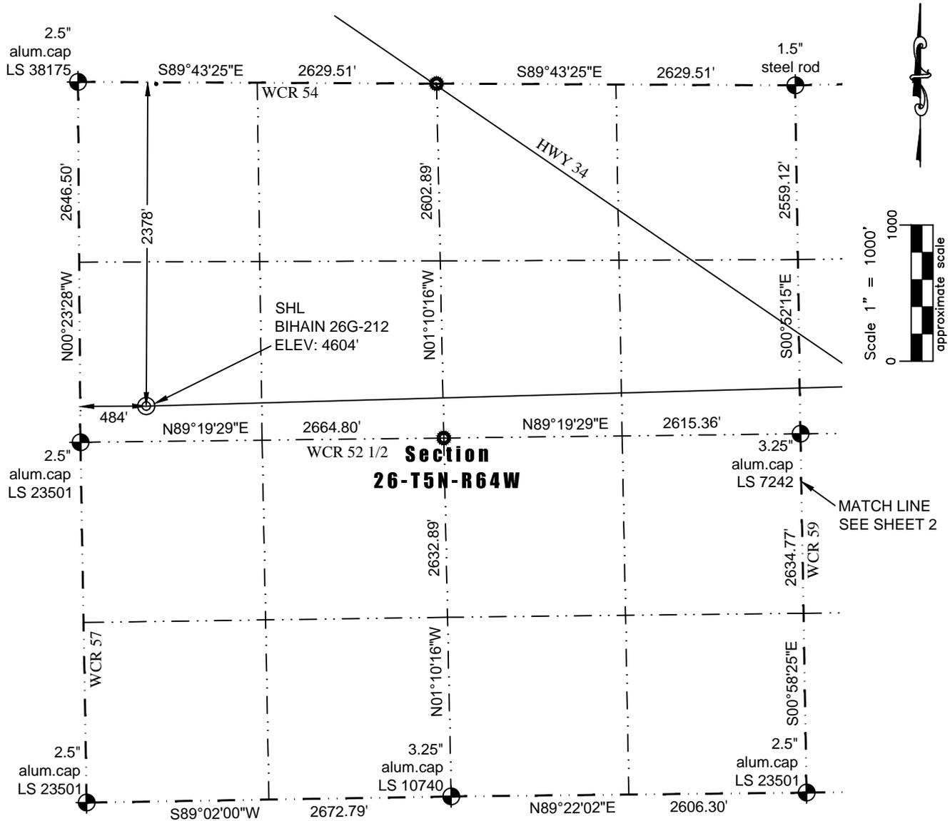
In accordance with a request from Barney Hammond of PDC Energy, Inc., Washburn Land Surveying, LLC has determined the location of the **BIHAIN 26G-212** well site to be SHL: 2378' FNL and 484' FWL, (BHL: 2200' FNL and 500' FEL), as measured at ninety (90) degrees from the section lines of Sections 26 and 25, Township 5 North, Range 64 West of the 6th Principal Meridian, Weld County Colorado.
