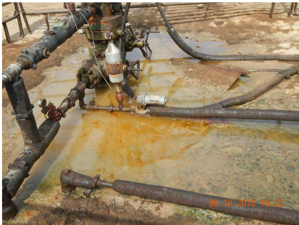
Sheen on fluid in Voloshin #3-25 cellar. Plywood debris in cellar.
