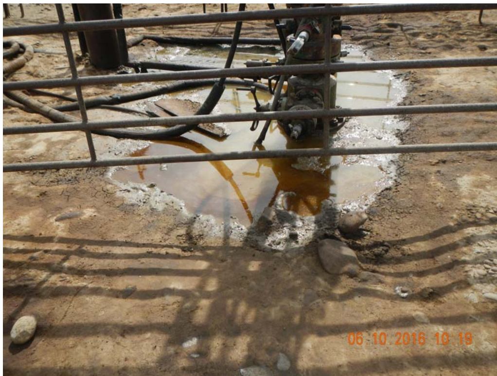
Voloshin #3-25 cellar filled with fluid with sheen on top. Stained soil around cellar perimeter.
