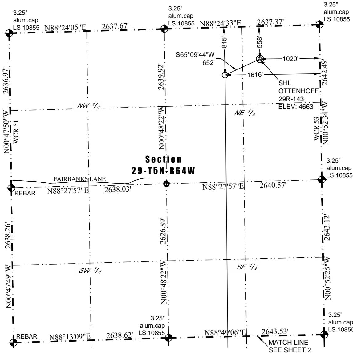
In accordance with a request from Paul Montville of PDC Energy, Inc., Washburn Land Surveying, LLC has determined the location of the **OTTENHOFF 29R-143** well site to be SHL: 558' FNL and 1020' FEL, (BHL: 2631' FSL and 1664' FEL), as measured at ninety (90) degrees from the section lines of Sections 29 and 32, Township 5 North, Range 64 West of the 6th Principal Meridian, Weld County Colorado.
