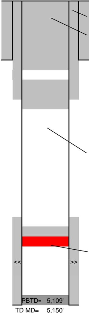
**Cut off casings 20' below GL and weld on marker plate w/ well name, number & API number.**
