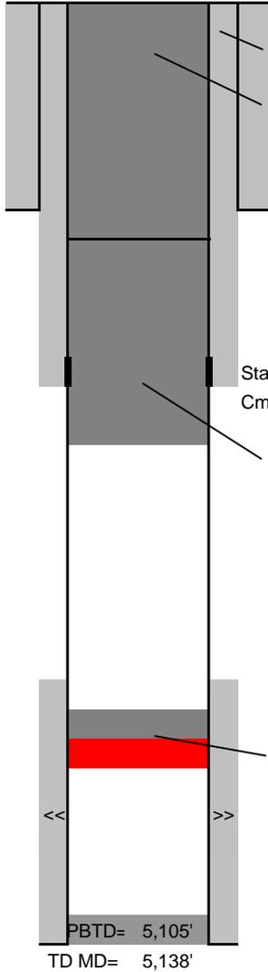
**Cut off casings 20' below GL and weld on marker plate w/ well name, number & API number.**
