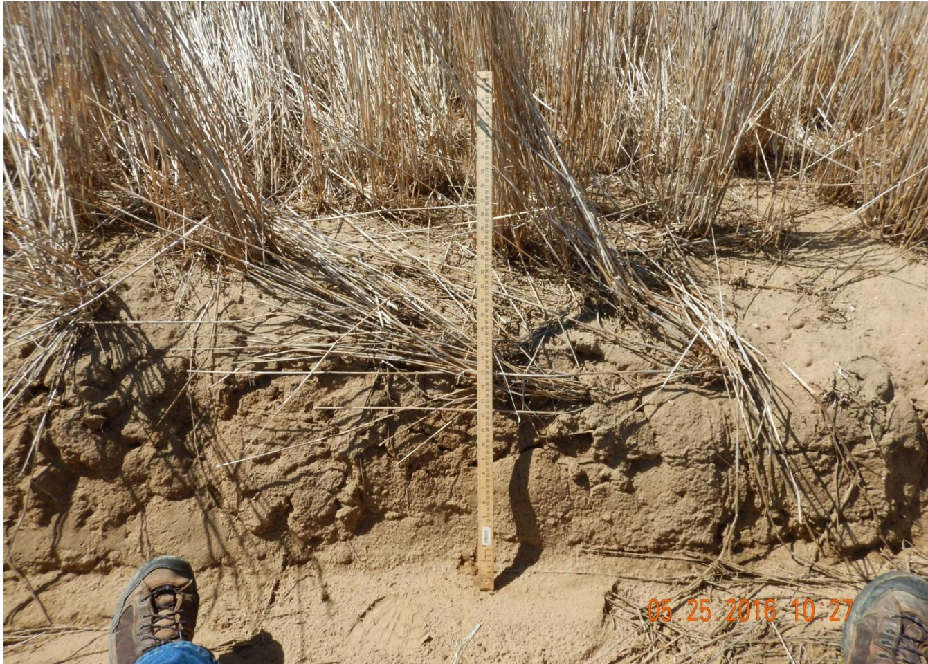
Photo 9. Photo taken from mid-way point of gully erosion measuring an average depth of 24".
