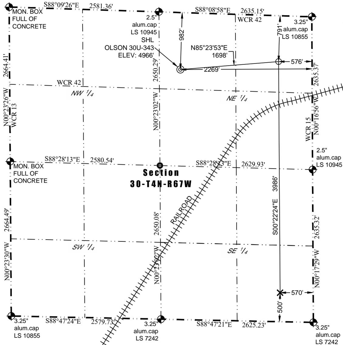
In accordance with a request from Mac Neumann of PDC Energy, Inc., Washburn Land Surveying, LLC has determined the location of the **OLSON 30U-343** well site to be SHL: 982' FNL and 2269' FEL, (BHL: 500' FSL and 570' FEL), as measured at ninety (90) degrees from the section lines of Section 30, Township 4 North, Range 67 West of the 6th Principal Meridian, Weld County Colorado.
