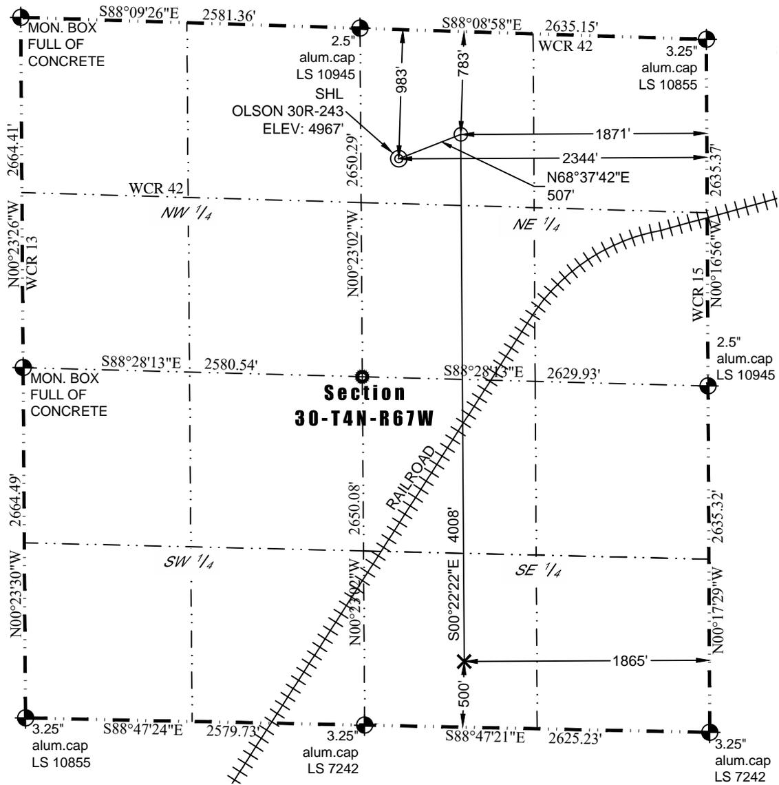
In accordance with a request from Mac Neumann of PDC Energy, Inc., Washburn Land Surveying, LLC has determined the location of the **OLSON 30R-243** well site to be SHL: 983' FNL and 2344' FEL, (BHL: 500' FSL and 1865' FEL), as measured at ninety (90) degrees from the section lines of Section 30, Township 4 North, Range 67 West of the 6th Principal Meridian, Weld County Colorado.
