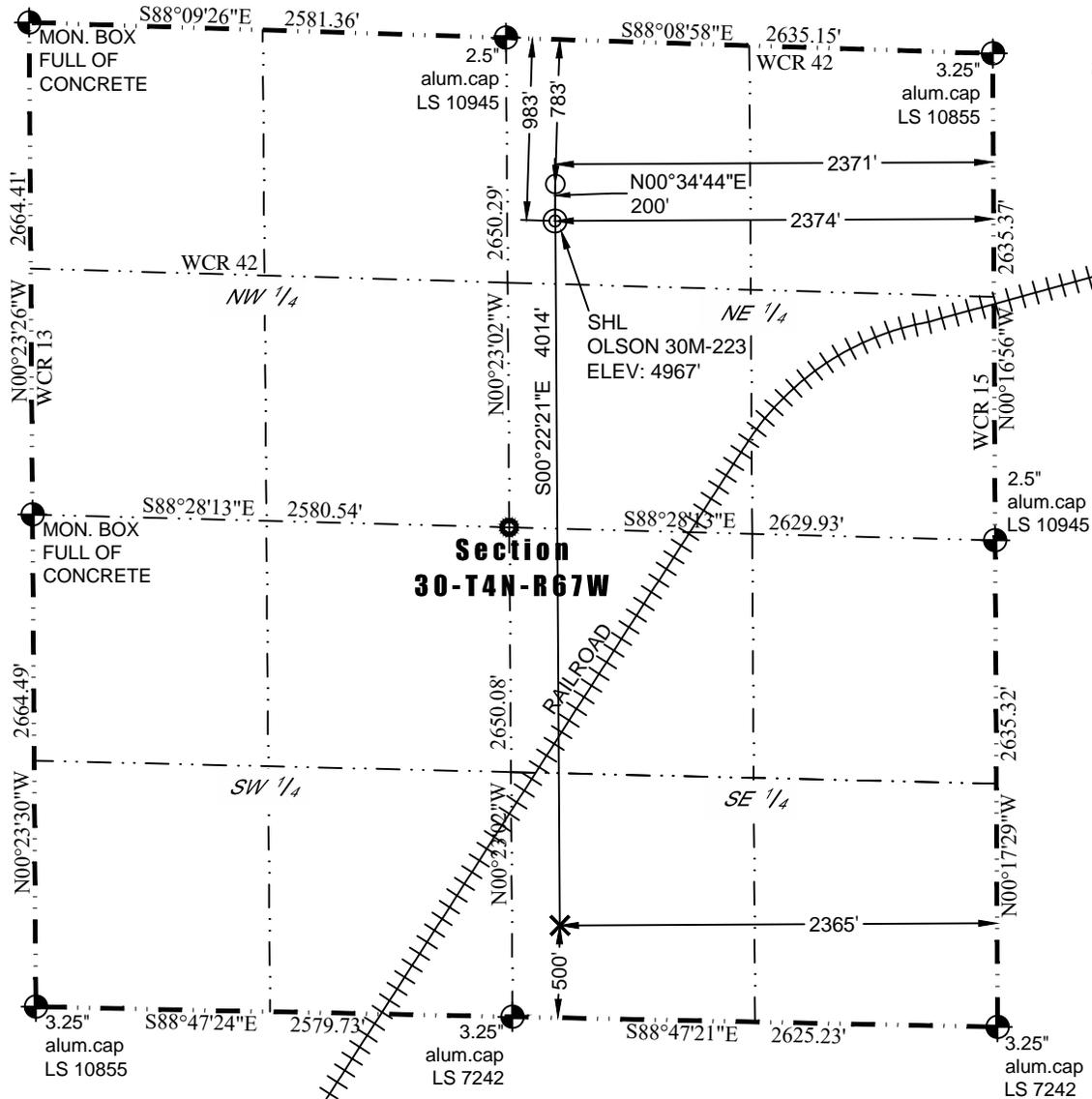
In accordance with a request from Mac Neumann of PDC Energy, Inc., Washburn Land Surveying, LLC has determined the location of the **OLSON 30M-223** well site to be SHL: 983' FNL and 2374' FEL, (BHL: 500' FSL and 2365' FEL), as measured at ninety (90) degrees from the section lines of Section 30, Township 4 North, Range 67 West of the 6th Principal Meridian, Weld County Colorado.
