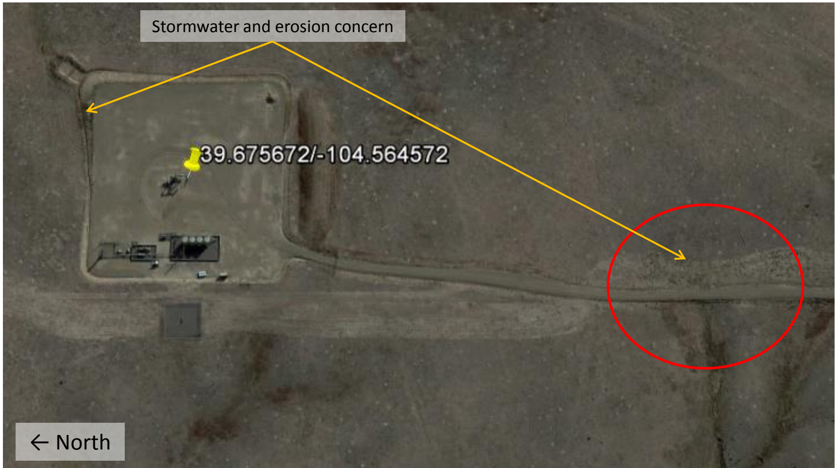
Photo 2. Google Earth aerial imagery taken 10/9/2015. Two areas of concern need to control stormwater and erosion. One area is located on the northeast well pad and the second area is approximately 800 feet south of the entrance on a pipeline.
