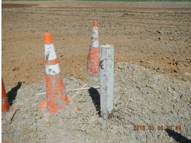
Monitoring Well #2 not secured.
