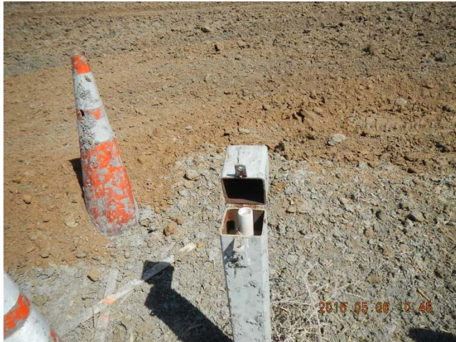
Monitoring Well #2 not secured.
