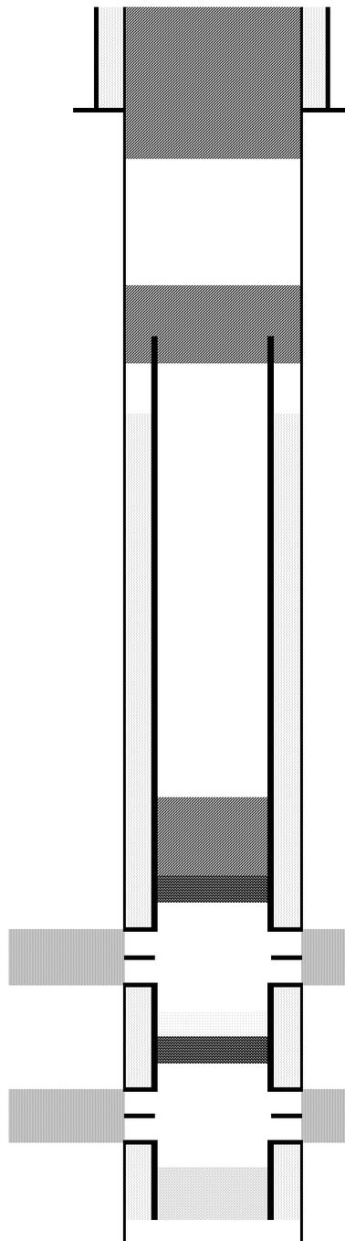
Cut surface casing off 6'-8' below surface.
