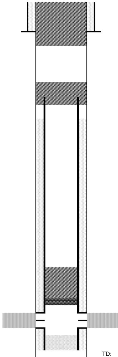
Cut surface casing off 6'-8' below surface.
