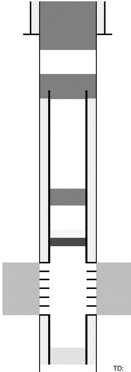
Cut surface casing off 6'-8' below surface.
