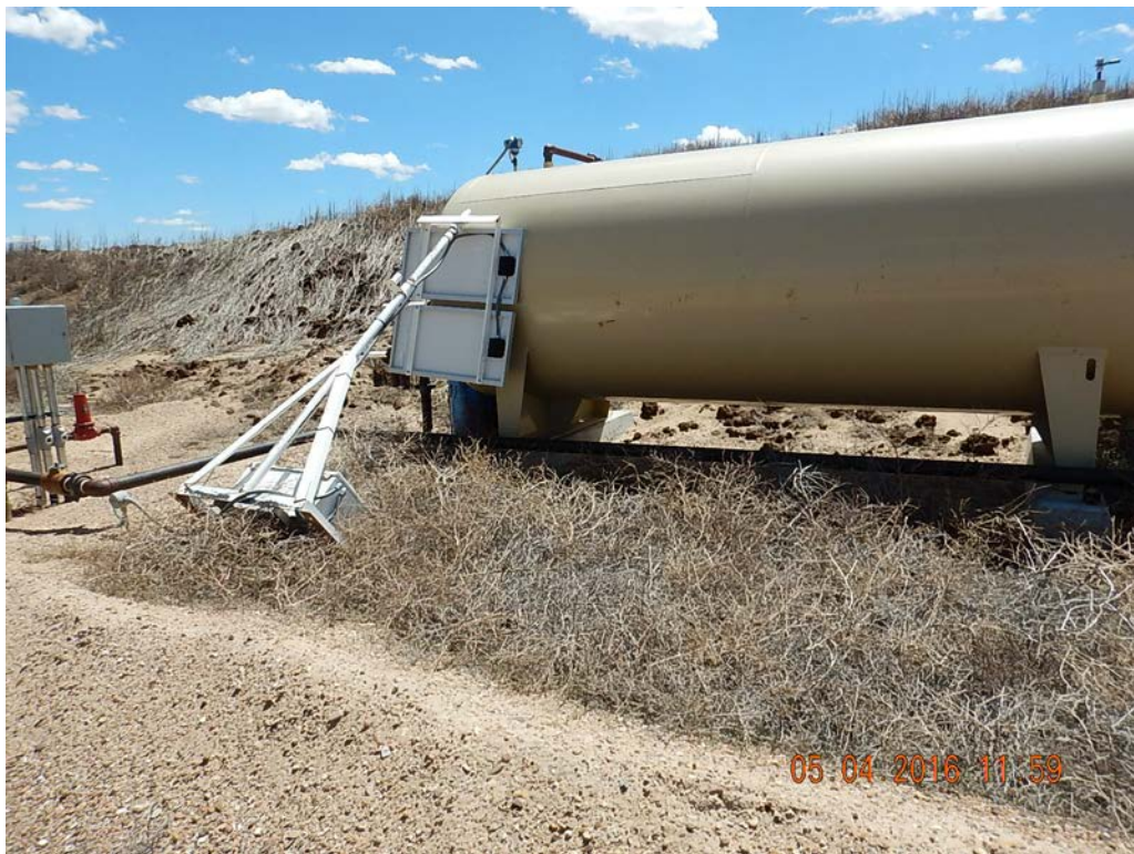
Figure 17 – Equipment fallen over and resting on tank.
