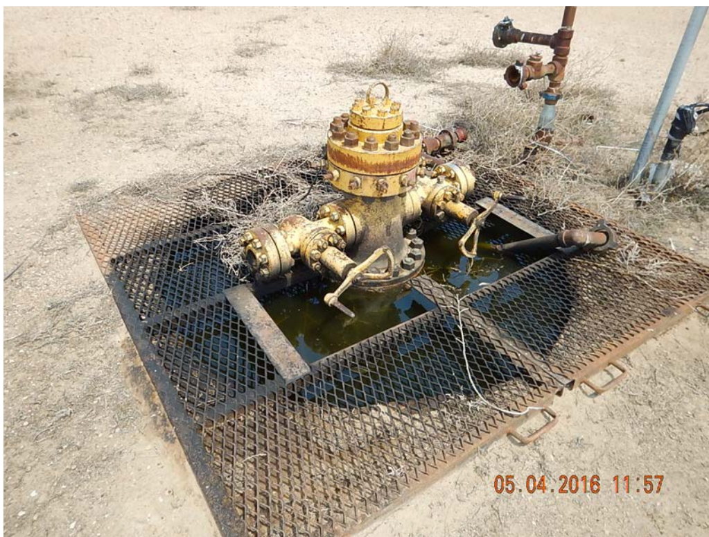
Figure 16 – Wellhead and cellar.
