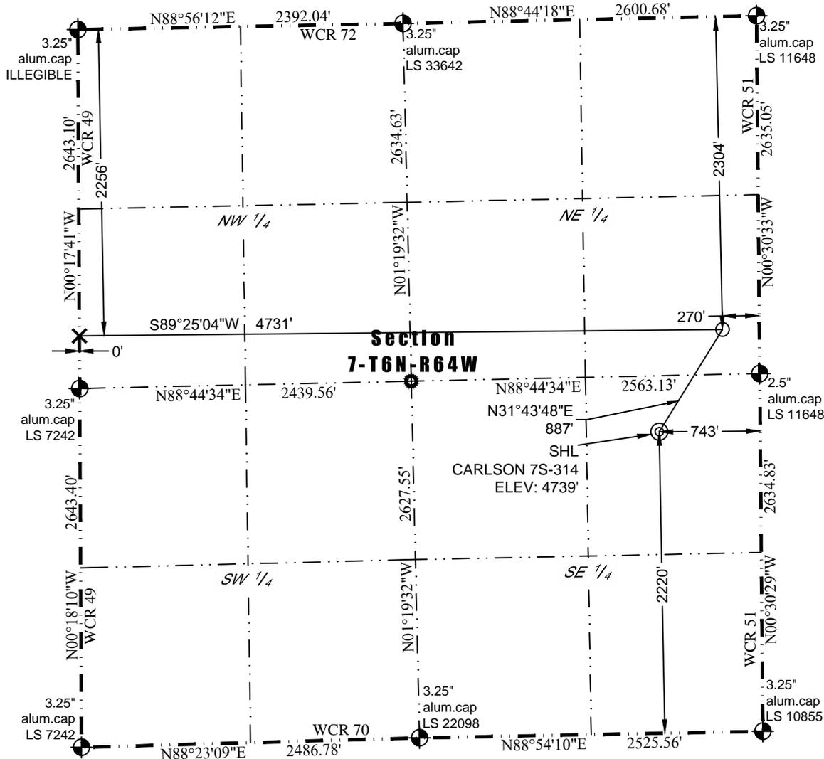
In accordance with a request from Barney Hammond of PDC Energy, Inc., Washburn Land Surveying, LLC has determined the location of the **CARLSON 7S-314** well site to be SHL: 2220' FSL and 743' FEL, (BHL: 2256' FNL and 0' FWL), as measured at ninety (90) degrees from the section lines of Section 7, Township 6 North, Range 64 West of the 6th Principal Meridian, Weld County Colorado.
