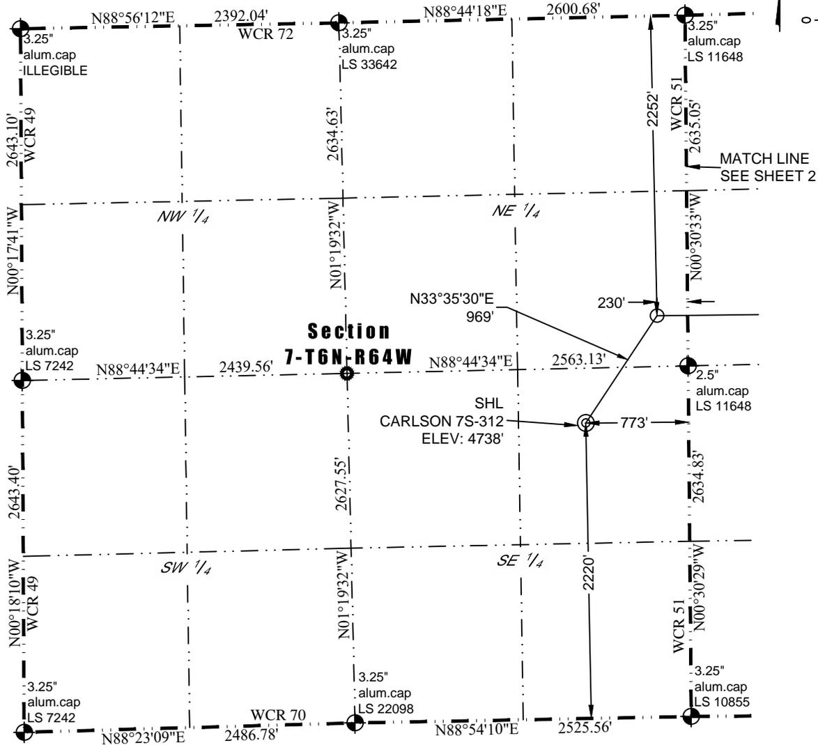
In accordance with a request from Barney Hammond of PDC Energy, Inc., Washburn Land Surveying, LLC has determined the location of the **CARLSON 7S-312** well site to be SHL: 2220' FSL and 773' FEL, (BHL: 2326' FNL and 500' FEL), as measured at ninety (90) degrees from the section lines of Sections 7 and 8, Township 6 North, Range 64 West of the 6th Principal Meridian, Weld County Colorado.
