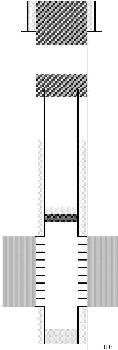
Cut surface casing off 6'-8' below surface.
