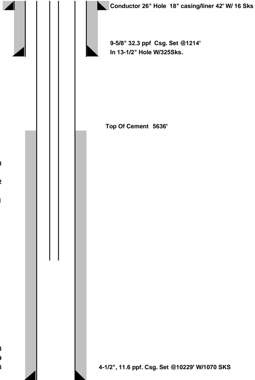
Conductor 26" Hole 18" casing/liner 42' W/ 16 Sks
